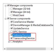
2. In the *Recorder Manager*, navigate to **Server** and select the correct Transcoding Module. Select the check box to associate the Device Manager for the Transcoding Module.
