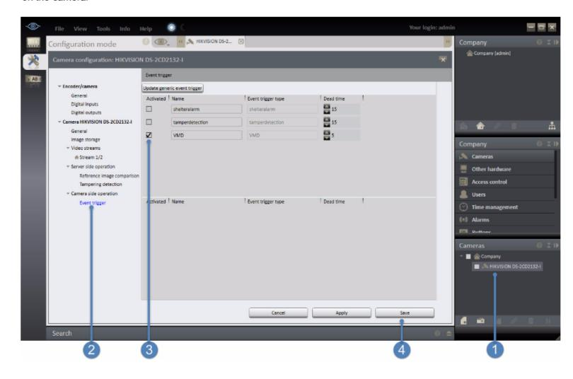
Log into Ocularis Recorder Manager and select the camera that will have motion detection enabled. (1)
